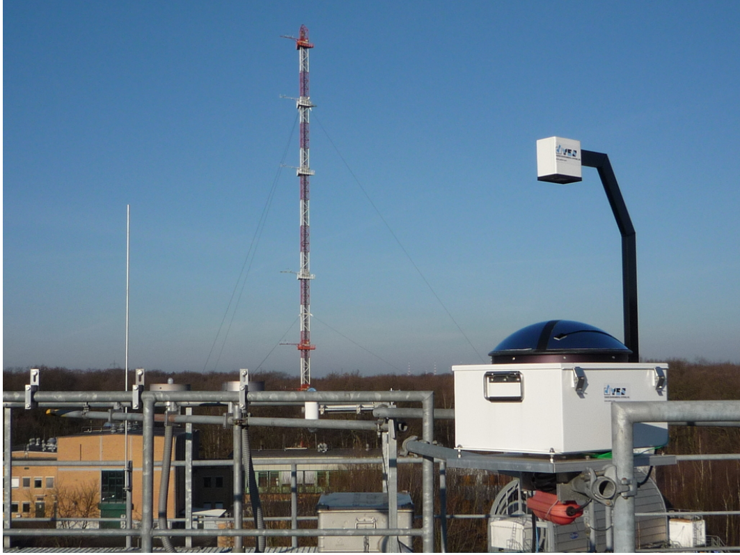
Figure 1: Setup of the total sky imager (TSI) on roof of institute ICG2 in the research center Jülich in front of the 120 m meteorological tower.
