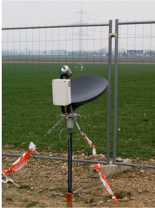
Figure 1: Setup of the MRR at site Selhausen.
