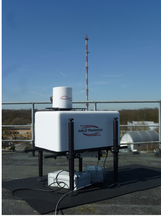
Figure 1: The Halo Photonics Streamline Doppler Lidar on roof of institute ICG2 in the research center Jülich in front of the 120 m meteorological tower.
