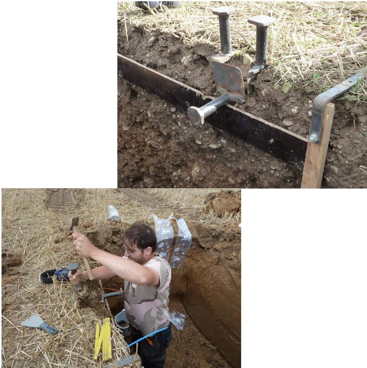
Fig. 9: Soil monolith sampling for the determination of the root length density. (source: A. Stadler)
