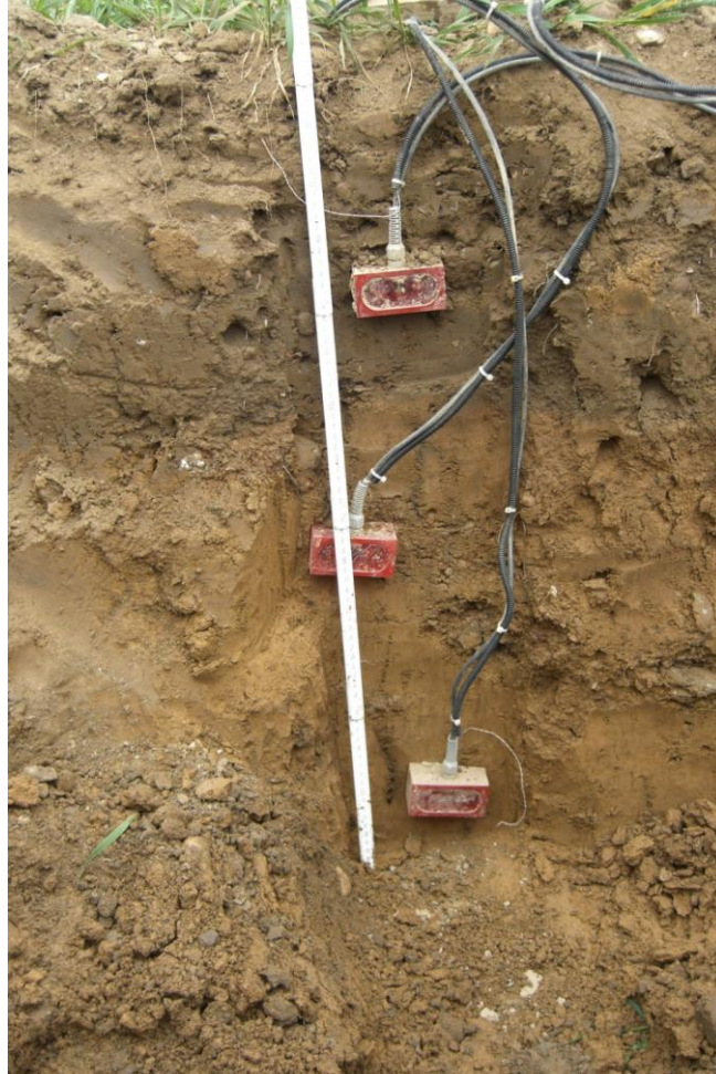
Fig. 11: TDR probes installed in the soil depths 15, 45, and 75 cm (source: M. Kupisch).
